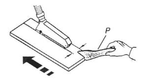
The push stick (p) serves as an extension of the hand and protects against accidental contact with the saw blade.
