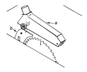
Installing blade guard (a) on riving knife (b).
